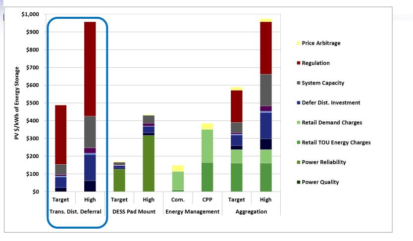
Substation can provide high value System Capacity and Regulation benefits. Transportable systems enable multiple, successive deferrals.
