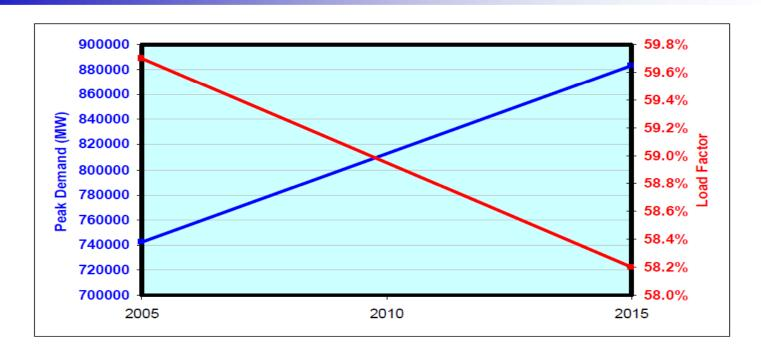
Peak Demand from 2006 to 2015 is Expected to Grow by 141GW and Load Factor to Decrease from 59.7% to 58.2%; Peak Demand Growth can be Levelized by Improving Load Factor to 69.2% in 10 years
