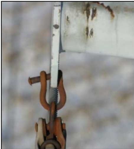
Rusted cathodic protection device insecurely mounted on a jack stand
